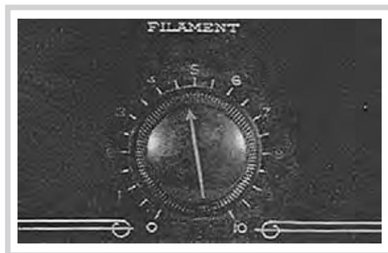
*Rheostats were used to maintain filaments at proper voltage as the battery ran down.*
