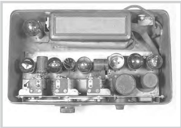
*Straight-down view of an AK 42. Power supply with 80 tube above; radio chassis with '26s, '27 and '71-A below.*
