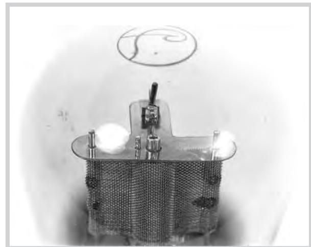
Note the cylindrical cathode emerging from the top of the UY-227’s interior structure.
