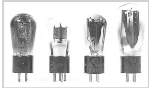
Here are the tubes that made the first true AC sets possible. From left: UX-226, UY-227, UX-171-A and UX-280.
