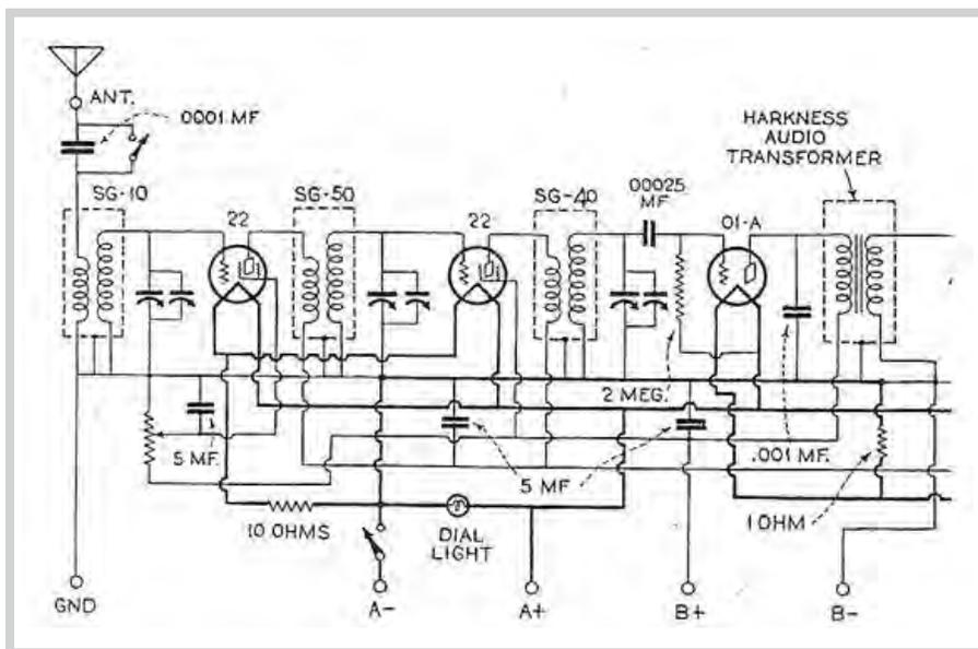
The “Harkness” battery-operated screen-grid set (1929) used type 22s as first and second RF amplifiers. Detector tube was the usual Type 01-A.
