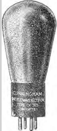
This full wave rectifier tube is equivalent to two single wave tubes, being constructed with two plates, or anodes, and two filaments. It is capable of giving an output of approximately 65 milliamperes, and is designed for use in "B" battery eliminators. It is capable of rectifying voltages up to 220 volts AC.
