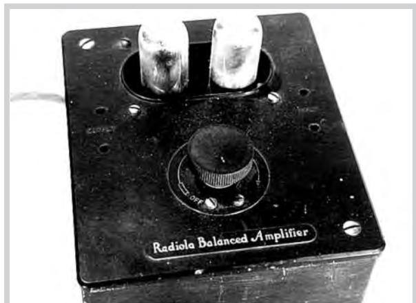
*The Radiola Balanced Amplifier was a desirable accessory for the Radiola III, enabling the little set to drive a loudspeaker.*
