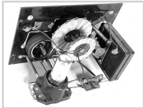
"Regen" sets could squeeze amazing performance out of one tube. Note pancake coils in feedback circuitry of a Crosley 50. The rear one is adjustable.
