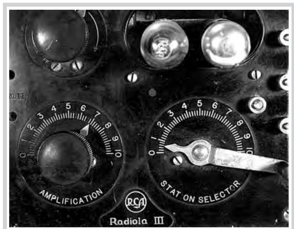
*Beside rheostats to control filament voltage, regenerative sets required only regeneration (“amplification”) and tuning controls.*
