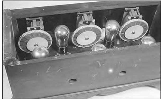
*TRF Circuitry required the use of three RF coils, each tuned by a separate tuning capacitor.*
