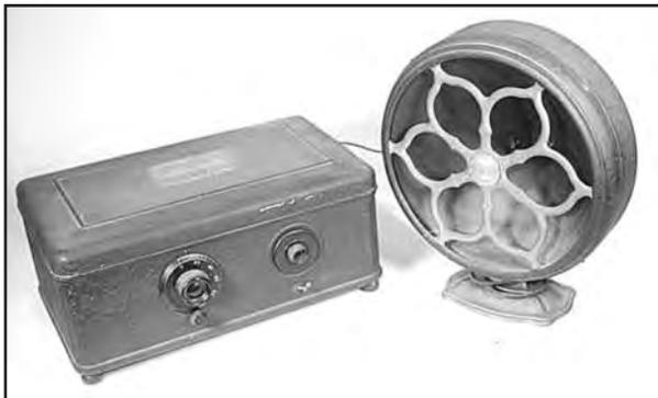
*The Atwater Kent Model 42’s simplified front panel, metal cabinet and square “footprint” typified the design of early AC sets.*
