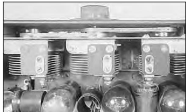
*Belting together the TRF's three variable capacitors made it possible to achieve one-knob tuning.*
