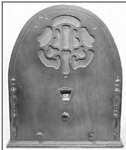
*The classic cathedral shape was formed when the side walls of the cabinet wall curved in over top of enclosed speaker.*
