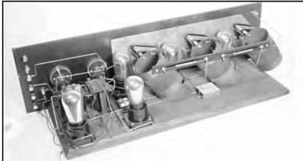
*1920s 3-dialer has typical breadboard-style “straight line” construction.*
