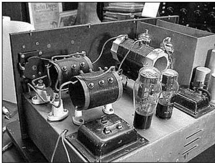
Interior view showing repaired antenna coils.
